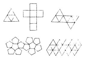
If the lines be cut with a sharp knife nearly through the paper, and the different plane surfaces folded at those lines and turned up, the edges will all meet and form the regular figures in order. The edges may then be secured by paste or glue.
