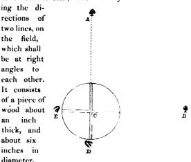
having two narrow slits cut with a saw at right angles to each other, and about half an inch deep. On the other side, a hole is bored with a centre bit, to a sufficient depth for placing it on the top of a pointed rod, which may be pushed in the ground when the lines are to be determined.
