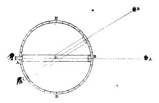
The whole will be obvious from the annexed figure in which ADBE is the divided circle, and AB the tube in imitation of a telescope.
