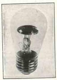
Figure 146. Argon-Filled Bulb for Showing Finorescence
