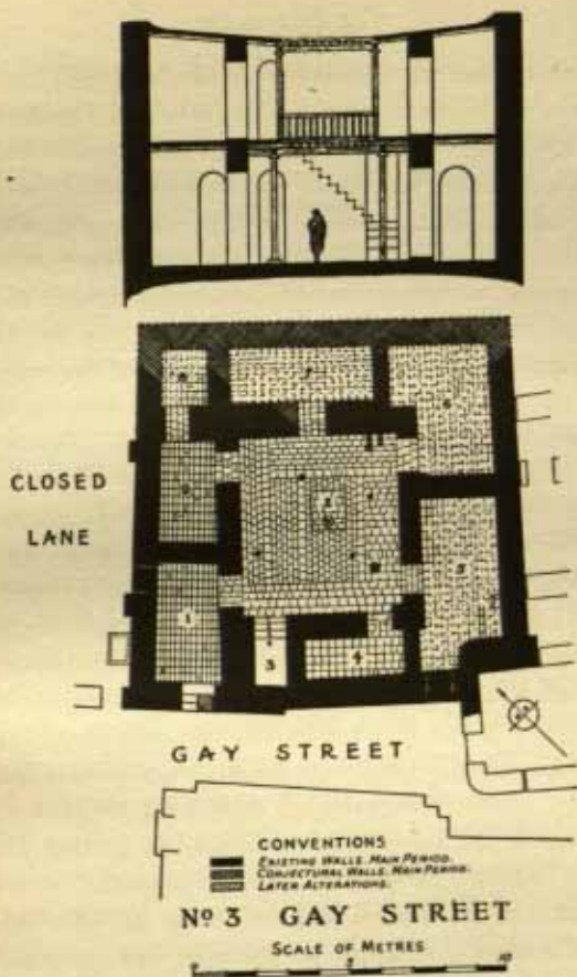
26. PLAN AND RECONSTRUCTION OF A PRIVATE HOUSE AT UR, OF THE PERIOD OF THE ISIN AND LARSA DYNASTIES
