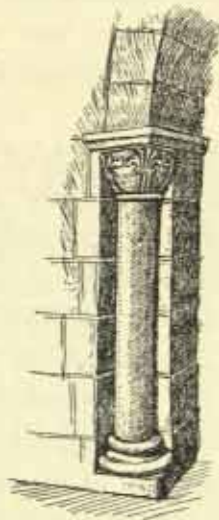
Fig. 6. Detail of Jamb of Fireplace.
