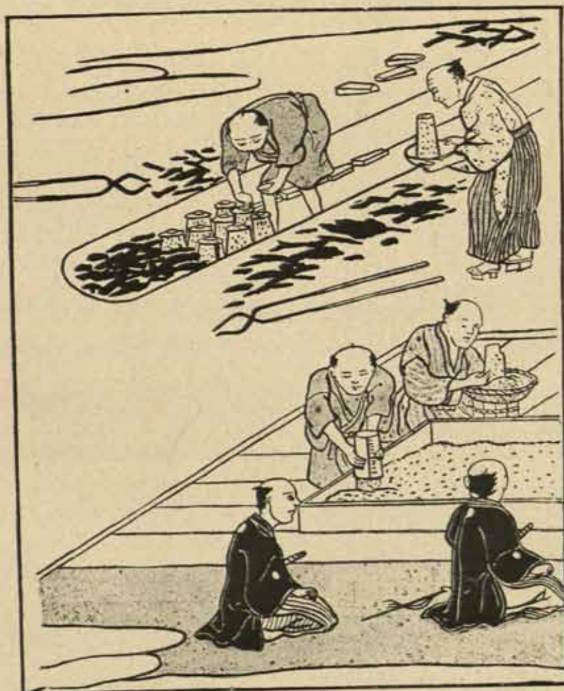
Fig. 3. Charging the furnace. Japan.
