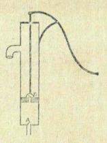
The suction pump, or atmospheric or lifting pump, consists of a cylinder called the barrel, with a valve A, in which works a piston or box in which is another valve B. Both valves open upwards. The piston is attached to a rod which is worked by a handle. When this is raised, the piston is depressed. The valve B then opens upwards allowing the water or air below it to escape into the upper part of the cylinder. When the piston is raised, the valve in it closes and
