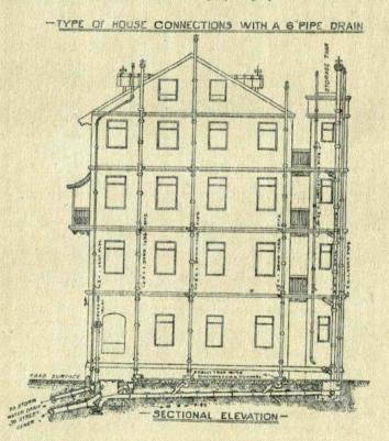
or cast iron bend. The gully-trap shall discharge into an inspection chamber fitted with a sewer trap as per Rule 5, or into a private pipe drain. The waste water pipes or nahani connections shall be constructed in accordance with Rule 23 for pipe drains.
