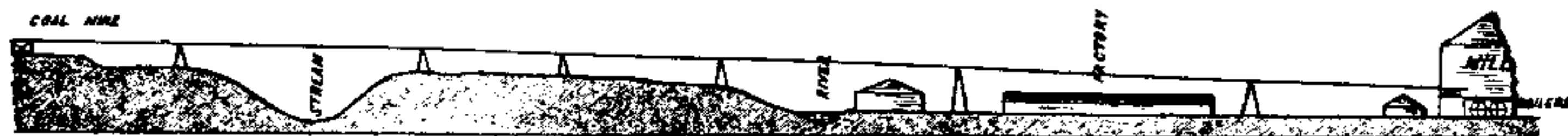
FIG. 58.—Installation of Wire-Rope Tramway at a Mill: Sectional Diagrammatical View.
