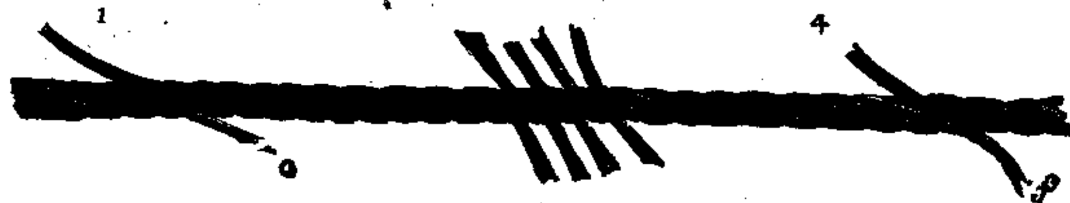
FIG. 79.—Splicing Wire Ropes: Second Operation.
