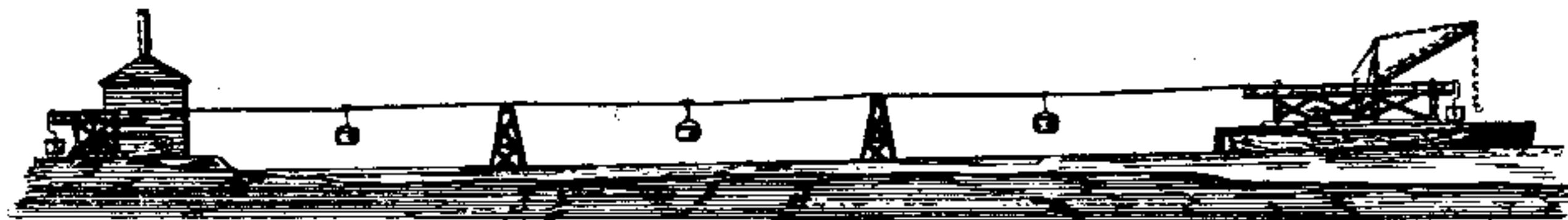
FIG. 50.—Installation of Wire-Rope Tramway arranged as a Pier.
