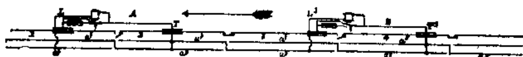
FIG. 30.—Blocking Arrangement for a Telfer Line with Minimum Interval equal to one Section of the Main Conductor.
