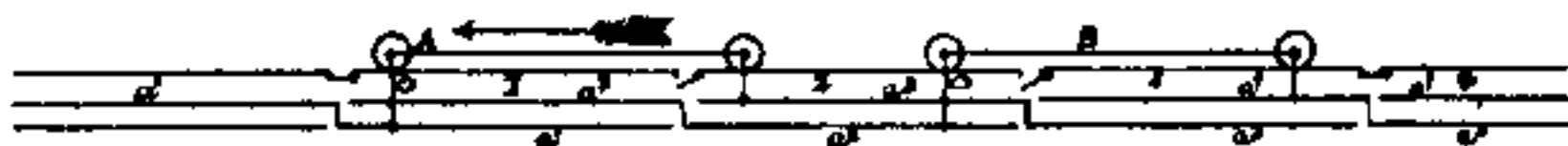
FIG. 31.—Blocking Arrangement for a Telpher Line with Inverted Block Wires and Cross Connections.
