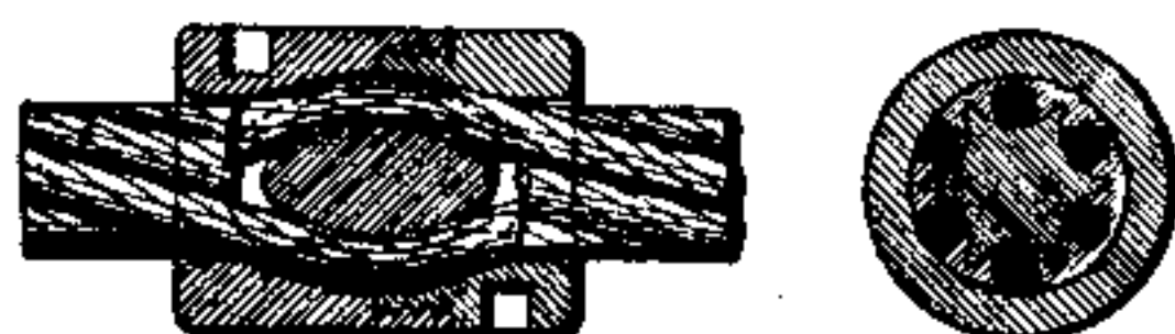
FIG. 12.—Modified Form of Otto Knot or Carrier Collar.
