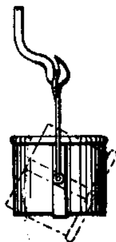
FIG. 19.—Tilting or Tipping Cylindrical Receptacle or Bucket.
