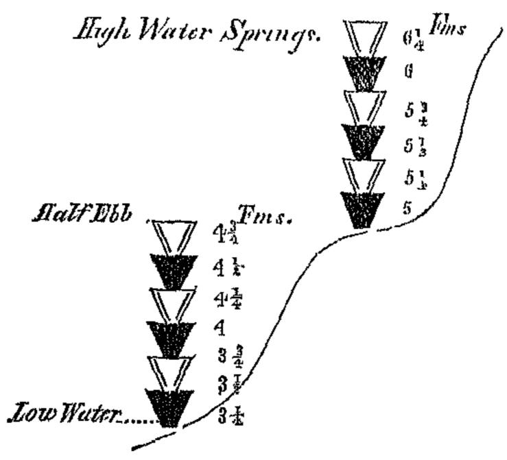
The Index Piles are not the same in all parts of the river, in some the notches are 12 inches, in others 18 inches, in length. (See River Surveyor's Reports) To tell the rise or fall of tide, is to deduct the number of notches appearing above water from those below.
