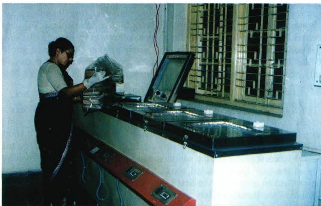
Operation of FREEZE DRIER in the Chemical Laboratory
