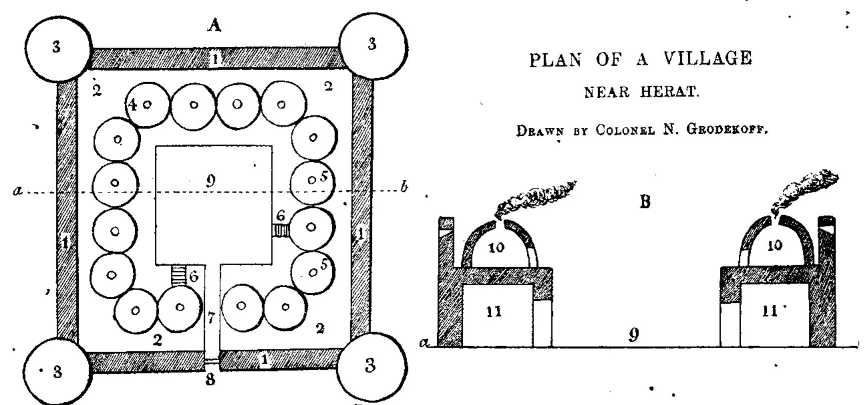
A.—Plan of the Village of Sheermas. B.—Profile along the line a b. 1.—Outer Wall. 2.—Roof of the Lower Storey, on which are placed a number of cupola-shaped Dwellings. 3.—Towers. 4.—Cupola-shaped Dwellings. 5.—Outlets for the Smoke. 6.—Staircase. 7.—Entry to the Village. 8.—Gate. 9.—General View of Sheermas. 10.—A Dwelling. 11.—Lower Storey for the Cattle.
