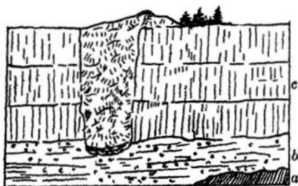
FIG. 5.—SECTION SHOWING RELATIONS OF BASALTS AND GRAVELS. STIKINE RIVER, EAST BANK, ABOVE TAHL-TAN.
