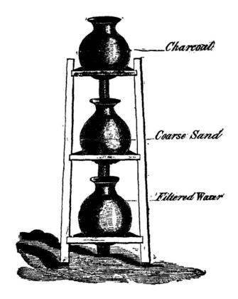
The local authority might, however, greatly improve the supply from public tanks by constructing filtering draw-wells in connexion with the tanks from which the water should be drawn by a pump or iron bucket and chain, after being filtered through gravel, coarse sand, and charcoal.
