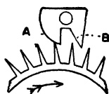
Fig. 47.—Escape Wheel and Pallets of Tictac Escapement
