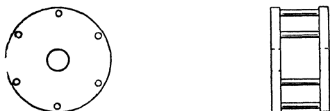
Fig. 6.—Two Elevations of “Lantern” Pinion
