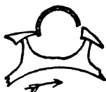
Fig. 43A.—Correct Locking of Teeth in Cylinder Escapement
