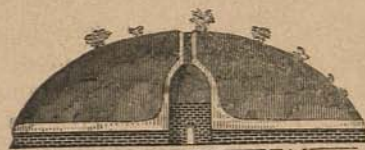
FIG. 17. SECTION OF TEMPLE-TOMB AT MOUNT ALVAN.
