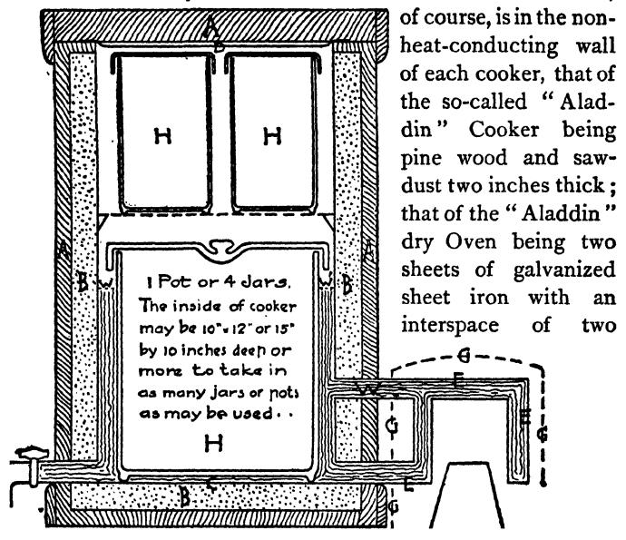
inches filled with carbonate of magnesia. In the oven which I used the interspace was only one and one-half inches, and it was not completely filled; I therefore wasted a good deal of heat.
