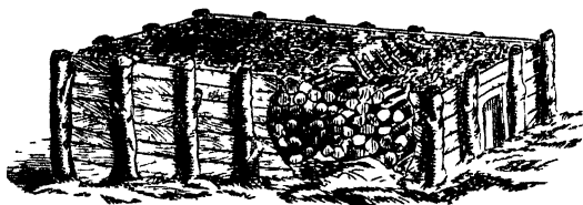
Fig. 5.—RECTANGULAR PILE FOR CHARCOAL BURNING.
