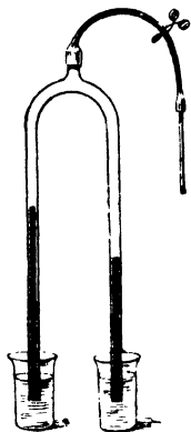
FIG. 45.- Hare's Method of Determining Density.
