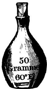
FIG. 43.—A Relative Density or Specific Gravity Bottle.
