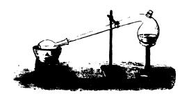
acid. Then put a lamp under the retort, and a flask, kept cool in a basin of water, to catch the acid which comes over. Soon a yellow liquid will collect in the
