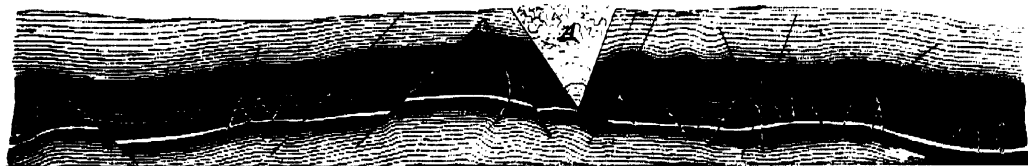
Trough Fault in Staffordshire Thick Coal.
