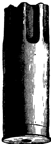
Method of Crimping the Kynoch "Perfect" Case with Greener's Corrugator.
