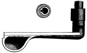
set on a false axis,\* the unequal revolution of which creates the slide. It thus presents no points for friction to wear off, and is quite another thing from a "cam," which is oval in shape, the extreme ends soon wearing.
