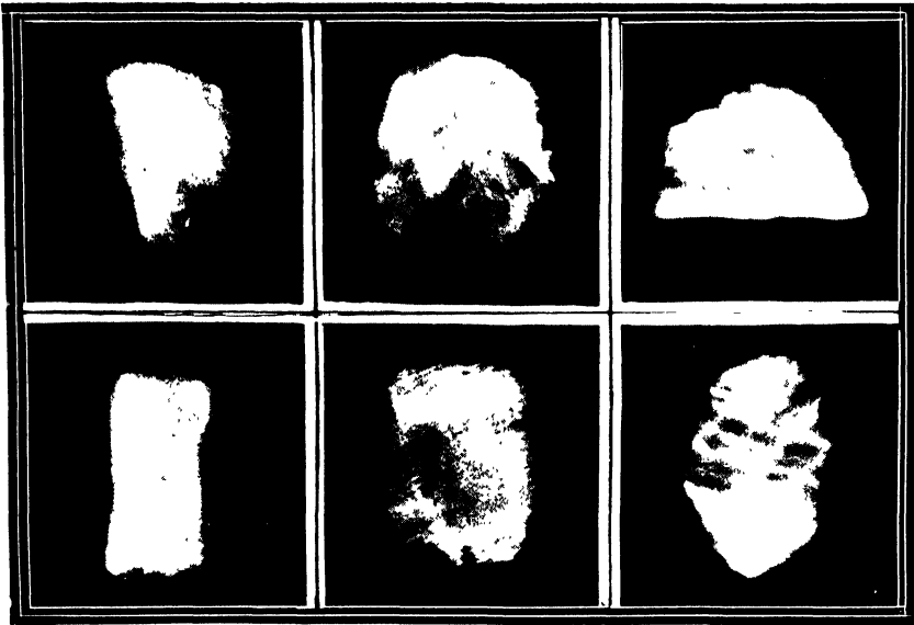
FIG. 6. X-Ray Topographs of Yellow-Luminescent and Non-Luminescent Diamonds
