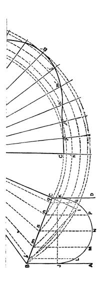
and w v. Then the trapezoid c v w d is the development of one of the planes forming the side of the roof covering.
