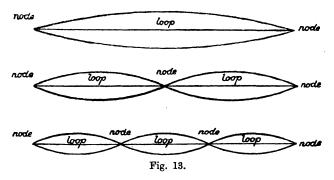
of a string, keeping its tension constant, we double its frequency of vibration and so raise its pitch an octave. This is easily verified by placing the movable bridge of the monochord under the mid-point of the string when either half of the string will be found to give the octave of the note given by the whole string.
