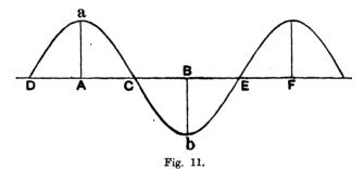
sented by lines drawn upwards from the axis of the diagram and backward displacements by lines drawn downwards, we shall then obtain displacement diagrams exactly like those we have been dealing with and shall be able to interpret them so as to ascertain what is happening to the various layers of air. Suppose for instance that Fig. 11 represents the state at a particular instant of air transmitting waves
