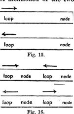
one fifth of the length of the pipe from the open end, the second three fifths from the open end and the third at the closed end. Now the frequency of the note given by a column of air in stationary vibration is, as in the case of the string, found to be inversely proportional to its length if vibrating as a whole.
