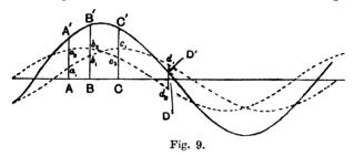
representing the displacements of successive drops at any instant would have exactly the same form, since the other drops in the line of propagation of the waves are all executing the same vibration and, at the instant in question, each shows a different stage of it. Thus the broken line may be taken to represent the form of the water surface at any particular instant, due to a system of waves. Now let the other broken line represent the form which
