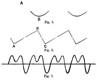
Fig. 5 represents the motion of a pendulum bob. It would be produced if the pendulum bob terminated in a pencil and were made to vibrate across a sheet of paper while the sheet was drawn sideways. We see that at A and B the line is parallel to the
