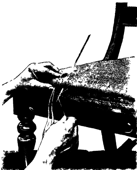
Fig. 59.—Stitching Second Row to form “Finger Roll”
