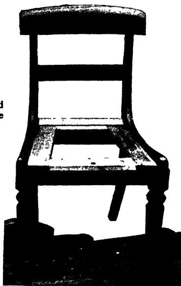
Fig. 49.—One Chair fitted with Loose Seat Frame for Upholstering
