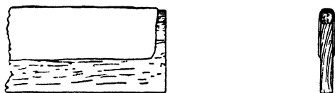
Fig. 124 and 125.—Method of Jointing Stringing on Upper Edge of Lining Slips
