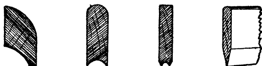
Fig. 7.—Rubber Blocks used in Glass-papering Mouldings
