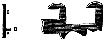
Fig. 121.—Mode of Repairing Pin of Back Spring Lock.
