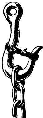
Fig. 137.—Mousing a Hook.
