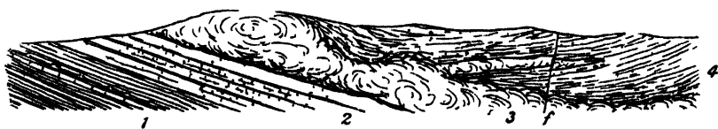
FIG 116 —Section of the bottom of the Midlothian Plateau, Linnhouse Water above Mid-Calder Oilworks
