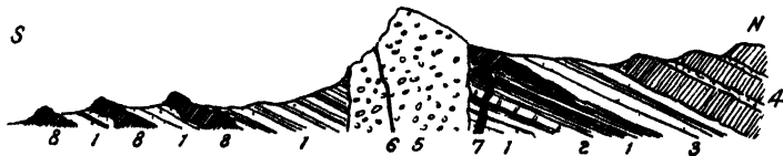
FIG 159—Section showing the position of the basic sills in relation to the volcanic series at Burntisland, Fife
