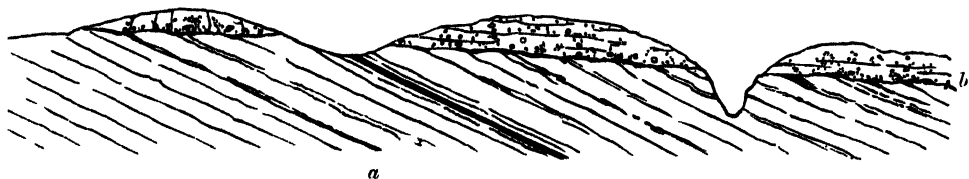
FIG. 208 — Section in brooks between Bonnytown and Balclastard, Largo a , Sandstone shales and coals of Carboniferous Limestone series b , unconformable tuff
