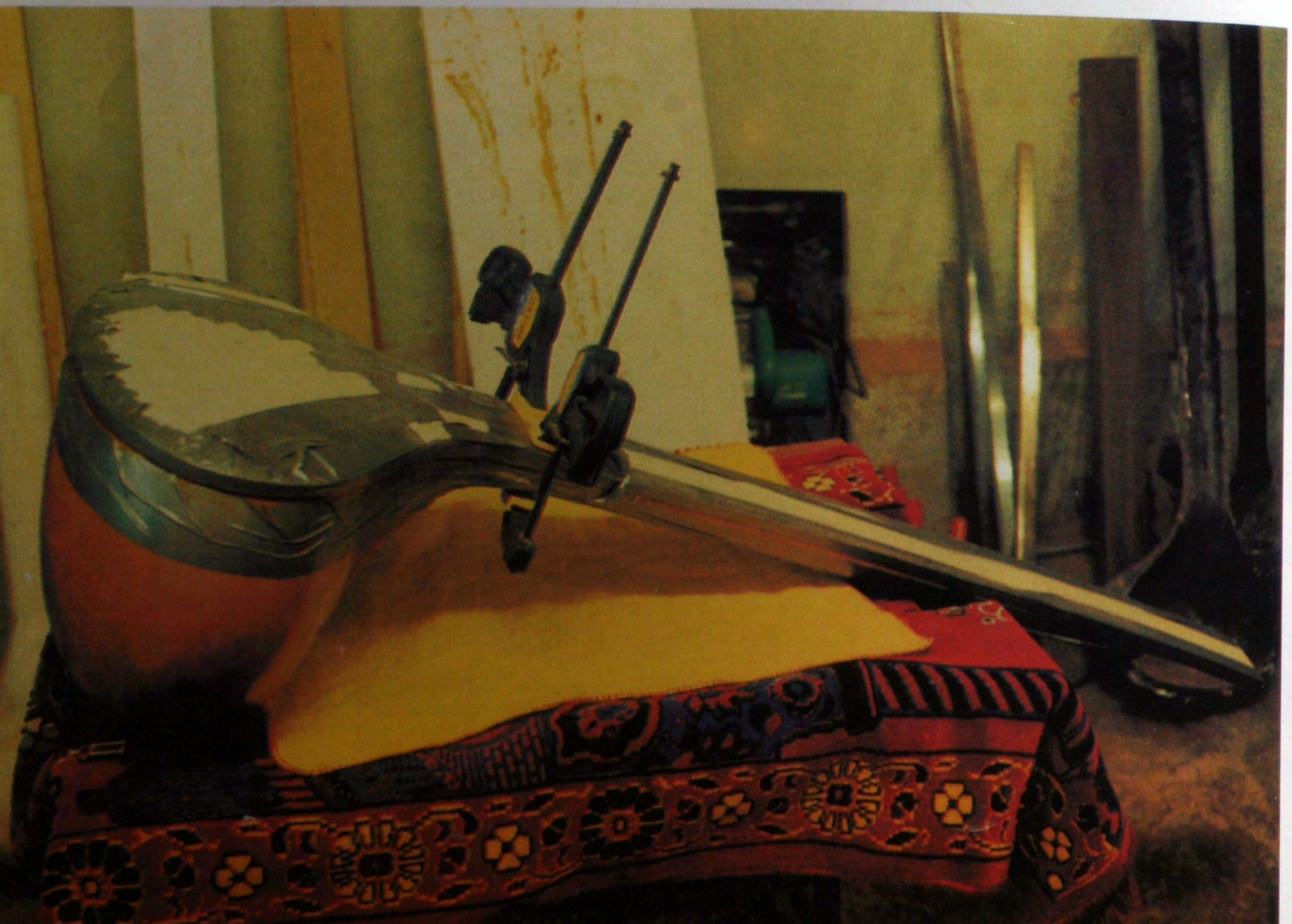
Fig. 2 ( above ): Paul van den Hout's one-piece Sitar body, combining resonator and stem, resting on the silicon mould from which it has been obtained. Fig. 3 ( below ): How van den Hout joins the tabli , neck heel, and finger-board to the one-piece resonator and stem of his Sitar.
