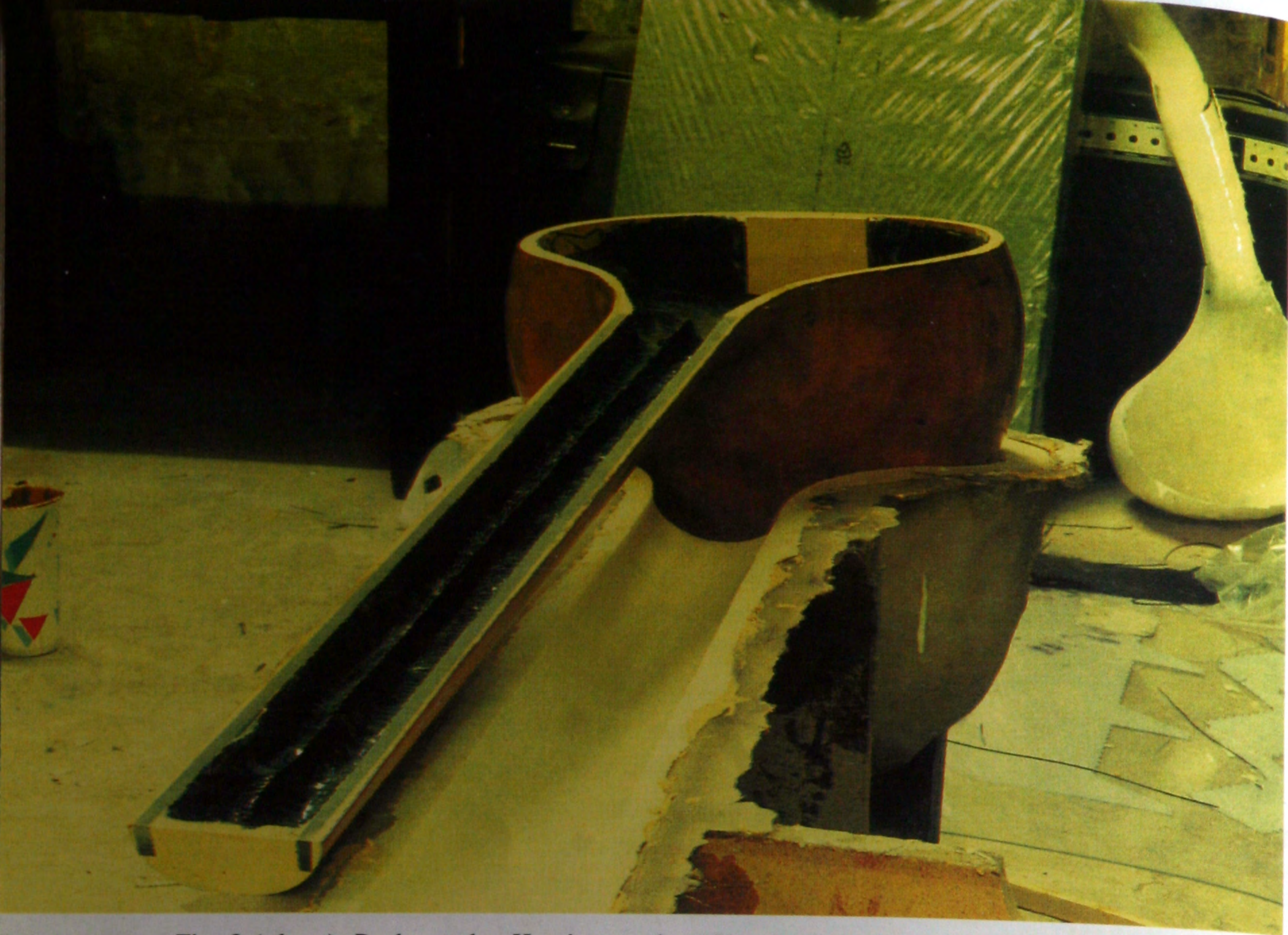
Fig. 2 ( above ): Paul van den Hout's one-piece Sitar body, combining resonator and stem, resting on the silicon mould from which it has been obtained. Fig. 3 ( below ): How van den Hout joins the tabli , neck heel, and finger-board to the one-piece resonator and stem of his Sitar.
