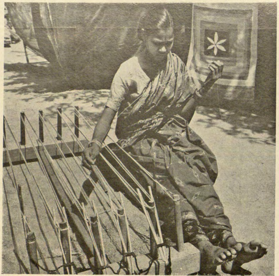
Plate 86 ▷ Preparation of warp, Village Tope, Bargarh area.
