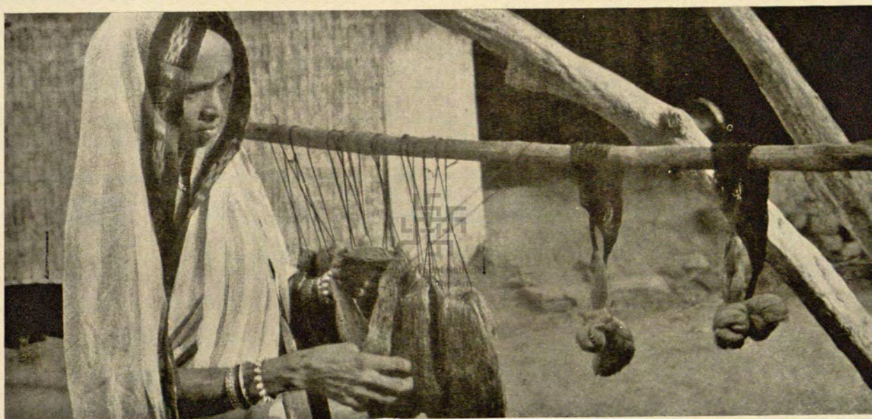
Plate 102 (bottom) Dyeing small spots by brush, Village Nuapatna.
