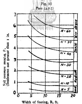
Chart based on water table not closer than B below base of footing. Fig: (c) Soil pressure corresponding to 1. inch settlement of footings on sand.
