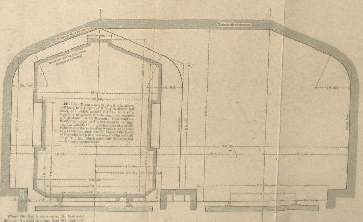
distance of a fixed structure from the centre of adjacent track is to be increased as follows:-
