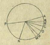
**197**. Let us suppose the sun and the moon to move in the same plane and in circular orbits, describing equal spaces in equal times. Let AB, BC, CD be the mean spaces described by the sun in three successive tithis, and let AM, MN, NP be the corresponding mean spaces described by the moon in the same tithis.
