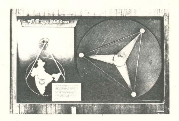
This model explains how communication through television is established around the Earth with the help of artificial satellites, such as 'Telstars', placed high above in the sky.
