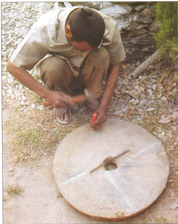
A blacksmith shaping a new grindstone for an updated water mill in the Himalayan state of Uttarakhand
