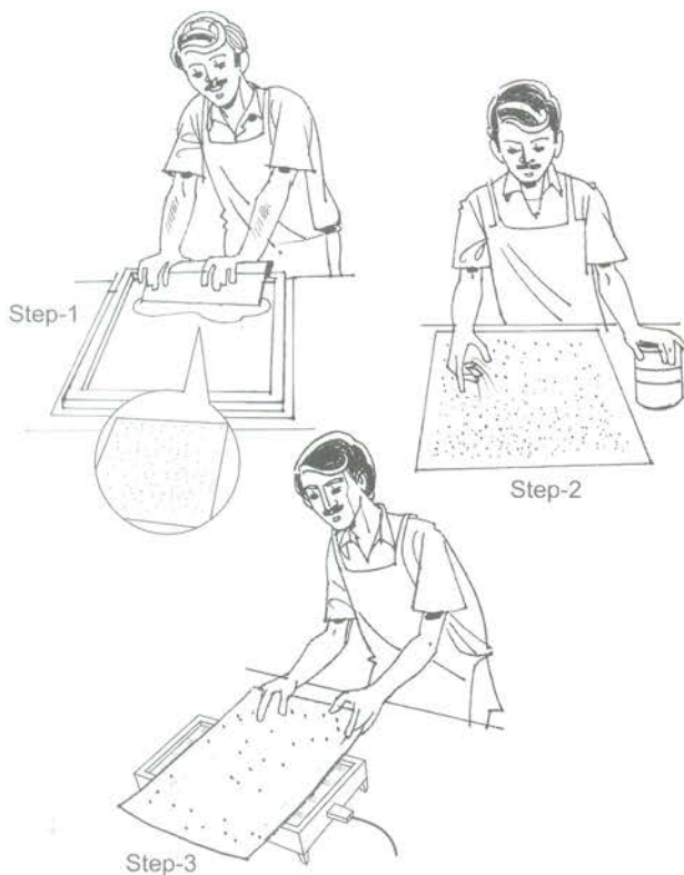
Fig. 14 The process of making raised dots on a metal plate
