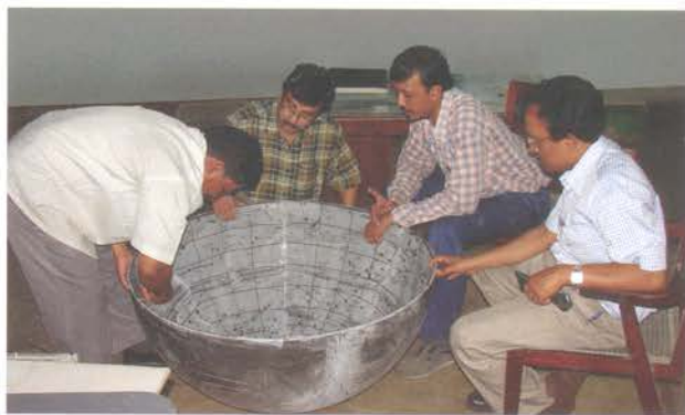
Fig. 10 In the making of a celestial hemisphere using reverse gores
